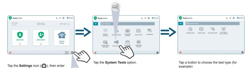
**Sensor Test:** Tests signals between the installed sensors and the Control Panel
