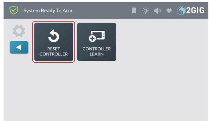
4. At the **Reset the Z-Wave Controller** screen, tap **Reset Controller**.
