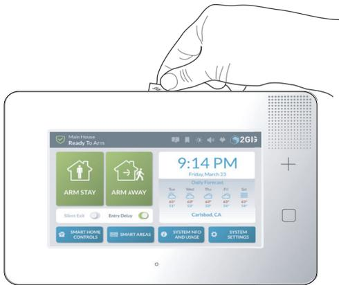
4. Insert a thumb drive storing the desired firmware version into the USB port at the top of the GC3 Panel.
