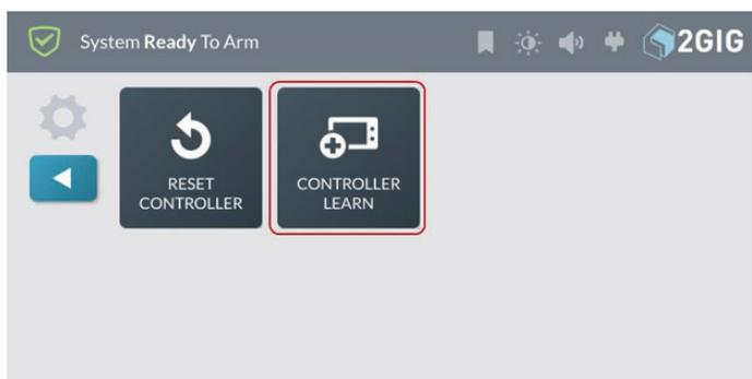
The GC3 Panel displays a “Learning Z-Wave Controller” message and waits for a signal from the primary controller. The synchronization takes time, depending upon the number of Z- Wave devices in the network.
