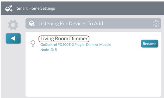
From the **Listening for Devices to Add** screen, you can continue by triggering the next desired device and then renaming it as needed.
