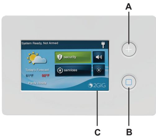
**A Emergency Button** (+). Displays Panic, Fire, and Emergency alarm activation (each has programmable options and can be enabled or disabled).
