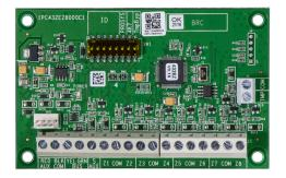
Adds an additional 8 hardwire zones to the Vario panel. Installs on the keypad BUS to accommodate remote mounting for easier wire runs. Includes an on-board tamper for installation in the 2GIG-VAR-ACCBOX.
