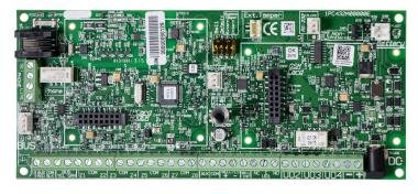
The Vario Main Panel Board offers install flexibility with features like, selectable bell output and case tamper, for enclosure door and wall. The Easy to install plug-in BUS header saves time in wiring. Each panel provides four programmable outputs, 1 NO/NC Dry Contact Relay and 3 programmable outputs.
