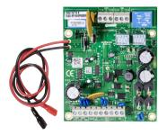
The power supply expansion module, providing total current capacity of up to 3 Amps with extensive remote diagnostics and supervision features, including tamper protection, over-current protection, two user programmable outputs and a dedicated siren driver.
